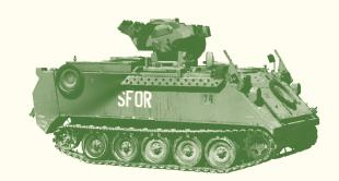
This variant of an armoured personnel carrier was used to carry out defensive and offensive engineering tasks. The M113 Combat Engineering Vehicle was fitted with a bulldozer blade and an auger. The bulldozer blade enabled the vehicle to push through obstacles, build defensive positions, or clear rubble from vehicle routes. The auger could be used to drill holes for barbed wire supports or to prepare sites for demolition.
